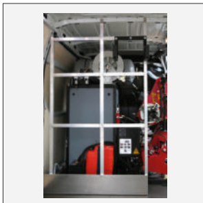
PROTECT YOUR EQUIPMENT ! H-shape separation in aluminium
