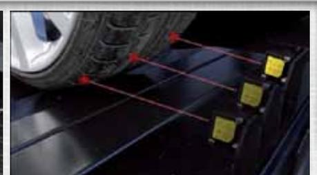
The profilometer is made up of **two reading units**, laser protection covers and relevant tyre centring runways.
