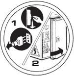
Unplug the power supply plug before performing any maintenance/repair operations on the machine.
