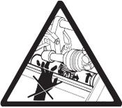
Never use the wheel spin shaft as a lifting point for the machine.
