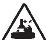
Hand-crushing hazard between rim and mounting head during mounting and demounting operations.
