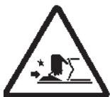
Hand-crushing hazard between rim and jaw during tyre locking.
