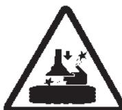
Do not place your hands on the wheel: when moving the arm to its working position your hands could be crushed between the rim and the mounting head.
