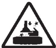
To prevent industrial accidents, keep hands and other parts of the body as far from the tool arm as possible when the table top is turning.
