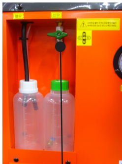
A valve to insert oil for oil replenishment
