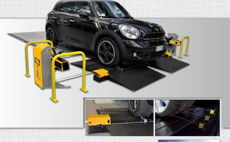
The profilometer is made up of **two reading units**, laser protection covers and relevant tyre centring runways.
